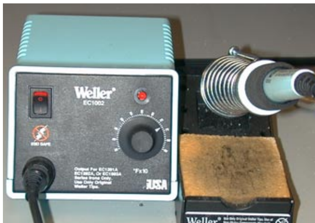
Figure 4. ESD safe soldering station with fine tip wand. This one is Weller model EC1201A
