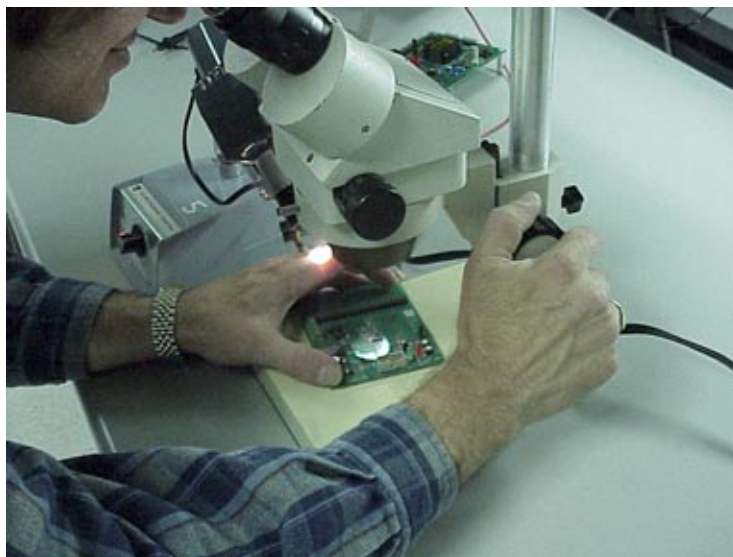
Figure 35. Stereo zoom inspection station (7X to 40X magnification) helps to inspect solder joint workmanship
