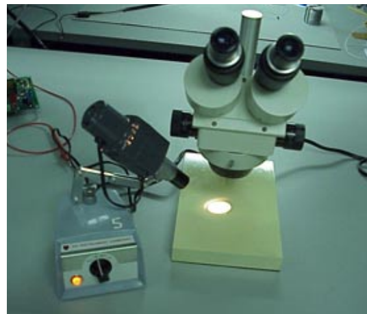
Figure 5. Optional equipment includes a PCB vise and an inspection microscope 7-40X
