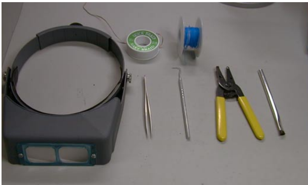
Figure 2. clock-wise from left: 4X magnifying headset, solder wick, wire wrap wire, stiff cleaning brush, wire strippers, and pointed tweezers
